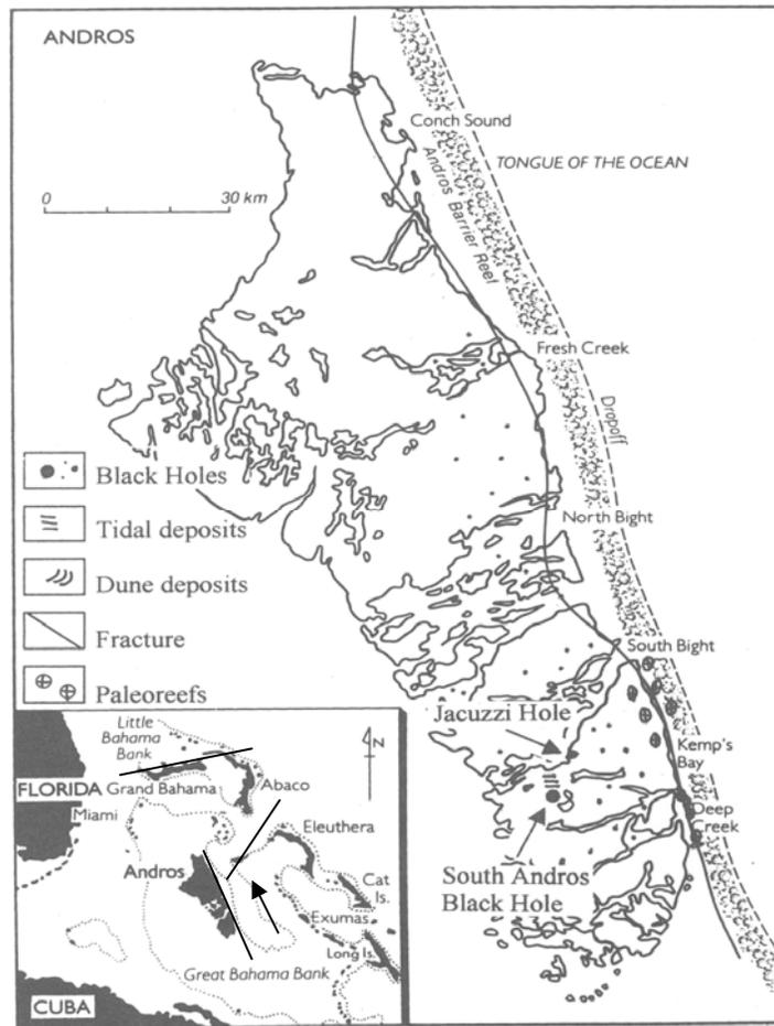
Figure 1. In the large diagram of Andros Island, on the east side of the island, it is possible to see that the cave openings (Paleoreef symbol) follow the fracture, as the fracture appears onshore and offshore. The smaller diagram in the lower left-hand corner is marked to generally show the direction of the fractures on Andros, Grand Bahama Island, and New Providence Island (arrow).
